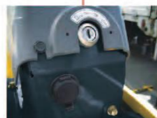
External Power Supply (12V)
